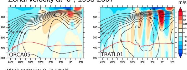
Black contours: O<sub>2</sub> in µmol/l Red countour: 27.0 kg/m<sup>3</sup> isopycnals
