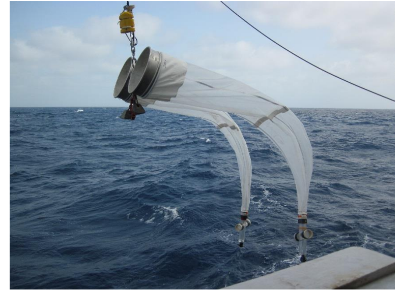
Bongo net (300 \mu m) from 200 m to the surface
